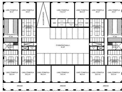
maantasokerros ja peruserkerros | ground floor and basic floor plans 1:1000
